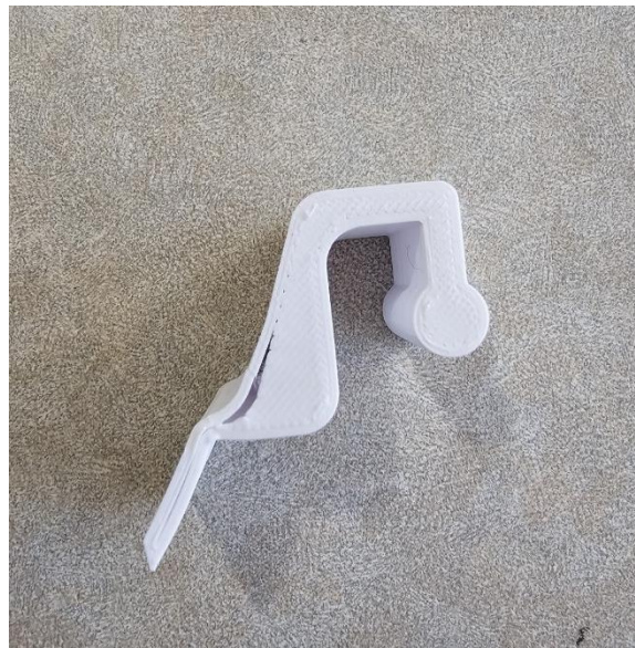
Fig 8.2.1: Mouthpiece after failure
