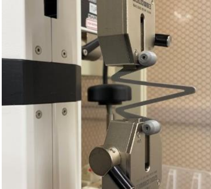
Fig 8.2.2: Spring at static position
